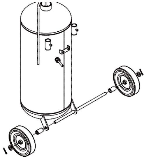
Step 1: Fit wheels, screws and scissor pins. # 16, # 15 and # 14.
