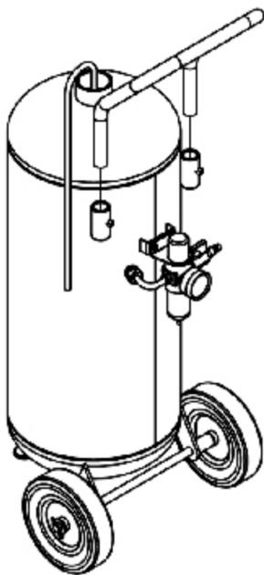
Step 4: Mount the handle (# 2) to the tank (# 1) with a screw (# 3).
