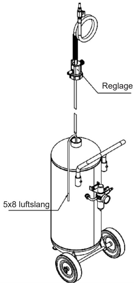
Step 5: Connect controls (# 23) to the tank (# 1).
