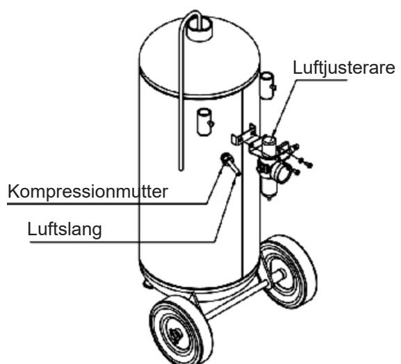
Step 3: Connect air adjuster (# 4) to the tank (# 1) using M5 screw (# 8), tighten with wrench. Connect air hose (# 10) to tank (# 1) with seal (# 11) and compression nut (# 12).
