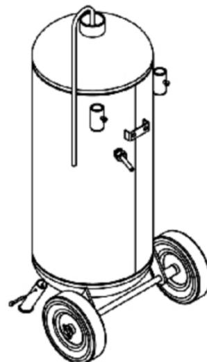
Step 2: Mount support legs with scissor pins. # 21 and # 22
