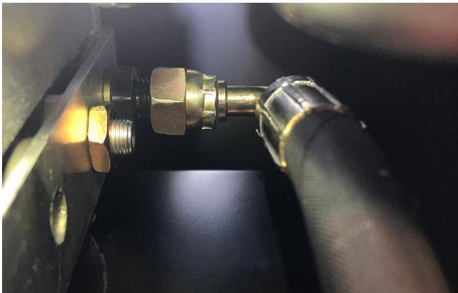
**Note:** Tighten the nipple on the pump housing firmly before mounting the hydraulic hose.
