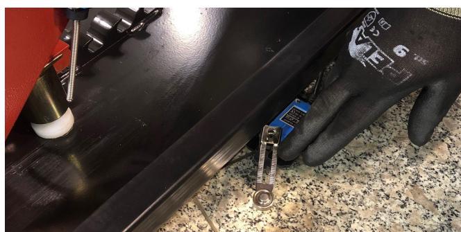
**Important:** Check that the sensor comes into contact with the beam.
