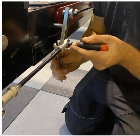
30. Fit the linkage and adjust the length so that all locks are released at the same time.
