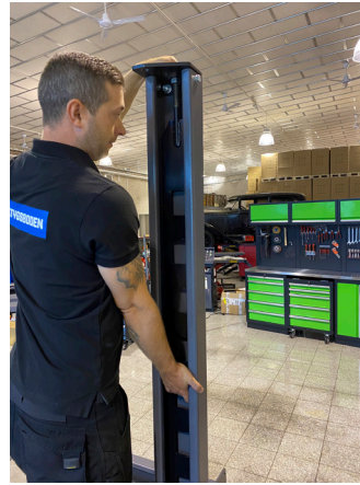
8. Attach the post cap check that the hole for the wire matches how the wire wheels are positioned. There should also be a nut with a washer on the crampton that should be on the underside of the cap.
