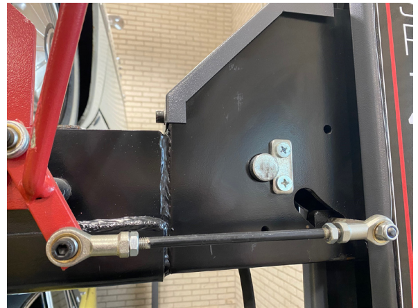
32. Raise the lifting ramps and place them on the bar at the same height in all corners. Adjust the latch steps if necessary and then tighten the wires.
