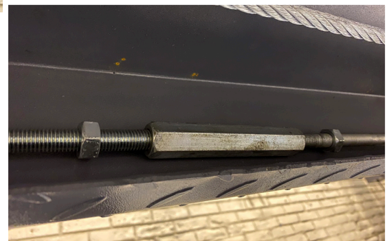
27. Mount the shaft to the latches remember to place the handle where the pump unit is located. Insert the other shaft from the other side and assemble them on the underside of the ramp.
