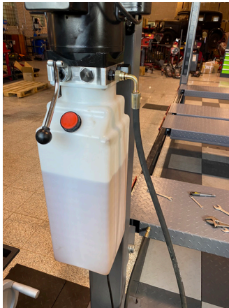
26. Top up with hydraulic oil. Fill to about 2-3 cm under the cap
