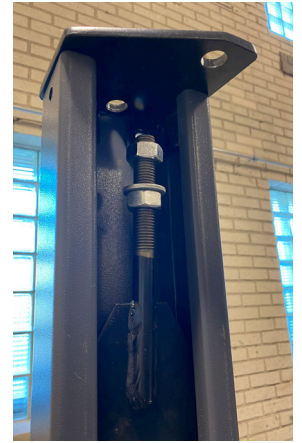
8. Attach the post cap check that the hole for the wire matches how the wire wheels are positioned. There should also be a nut with a washer on the crampton that should be on the underside of the cap.
