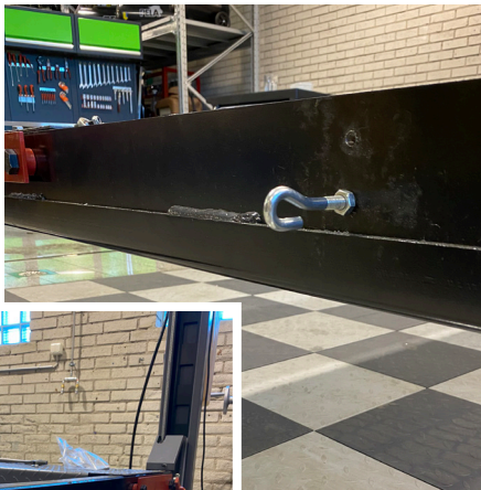
30. Fit the linkage and adjust the length so that all locks are released at the same time.
