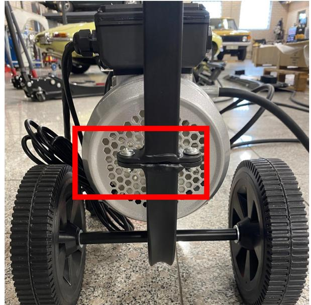
Mount on the handle with the included two screws, nuts and washers.
