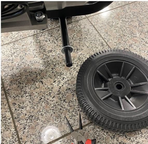
Mount on the wheels. First place the washer on the wheel axle, then the wheel with the concave side outwards. Attach then the wheel with the locking ring.
