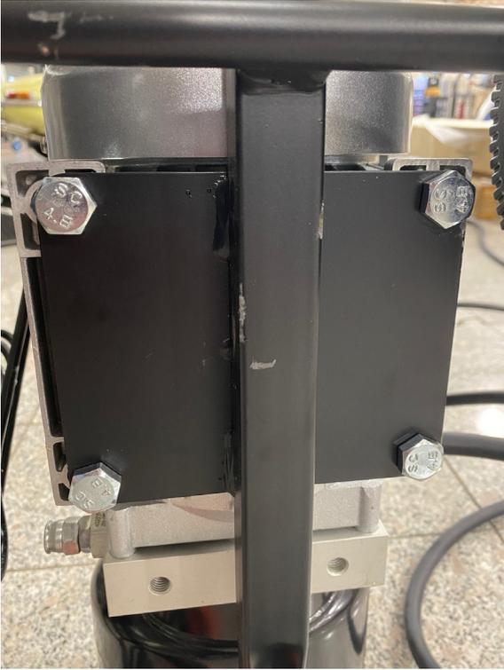
Mount the plate with wheel axle and socket for handles on the back of the pump unit. Use the supplied 4 screws and nuts.
