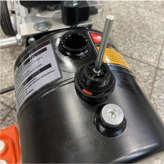
Fill the hydraulic tank with approx. 4 liters of hydraulic oil, VG32.
