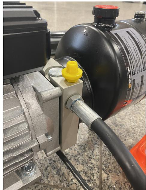
Remove the yellow plug from the pump housing and attach the hydraulic hose. **Check that the gasket is not stuck on the plug.** Tighten properly.
