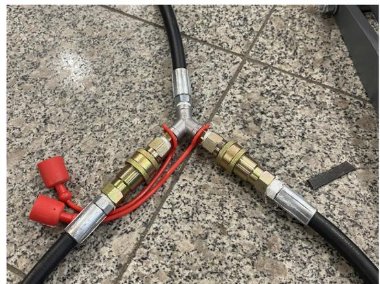
Connect the hydraulic hose to the two lifting ramps with the quick couplings. **Check that it fits properly.**
