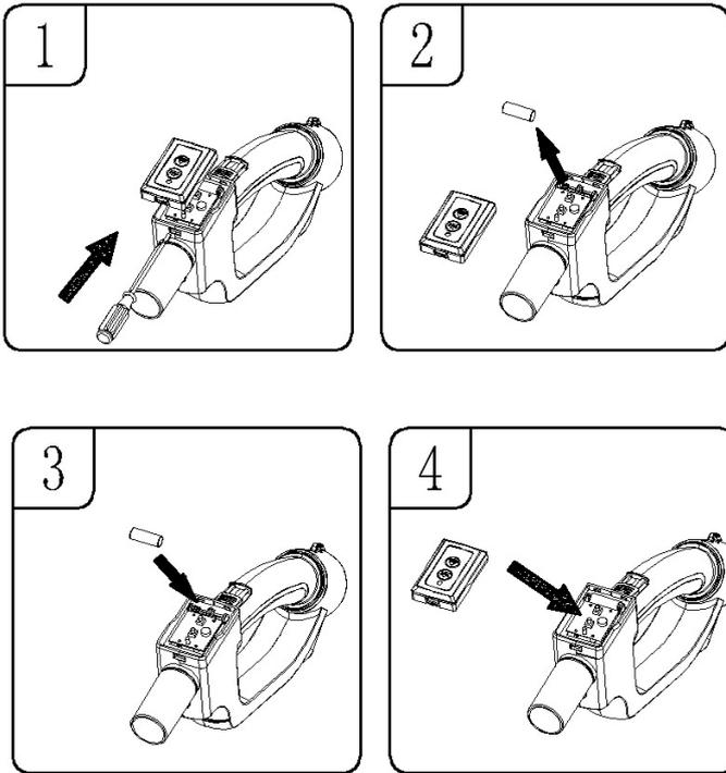
1. The battery cover can be opened by pressing the front of the battery box with a screwdriver. (Fig 1)
